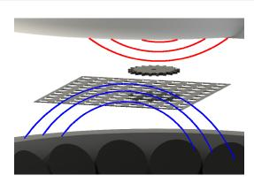
The gripped object is levitated in the low pressure regions of a non-audible acoustic field, as shown in the figure on the left. By using arrays of small sound transducers, the distribution of this field, and thereby the position and forces acting on the object, can be manipulated with high precision.
